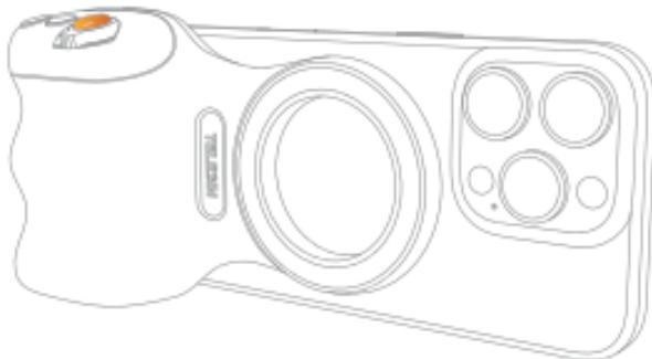
2. Power on by holding shutter for 2s, connect via Bluetooth TELESIN\_MG2. Auto shut-off if not connected within 2 mins.
