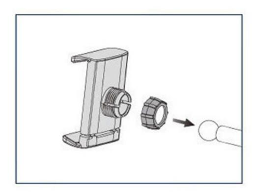
2. Slide screw cap over ball-joint head. Insert ball-joint head into holder socket. Fasten screw cap.
