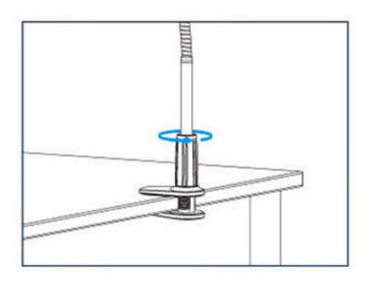
1. Adjust height of clamp then rotate clockwise to fasten.
