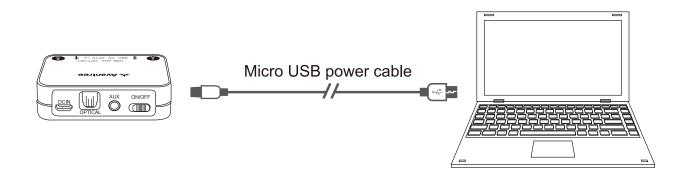
**Note:** The connecting cable must have both DATA SYNC and charging capabilities.
